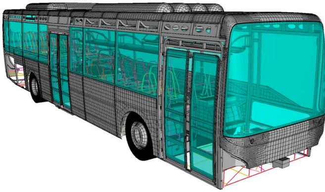
**FIGURE 1:** FEM model of bus
