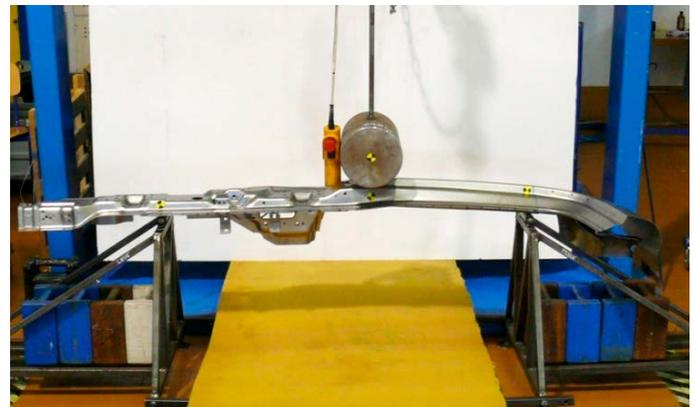
**FIGURE 5:** Drop test of an A-pillar
