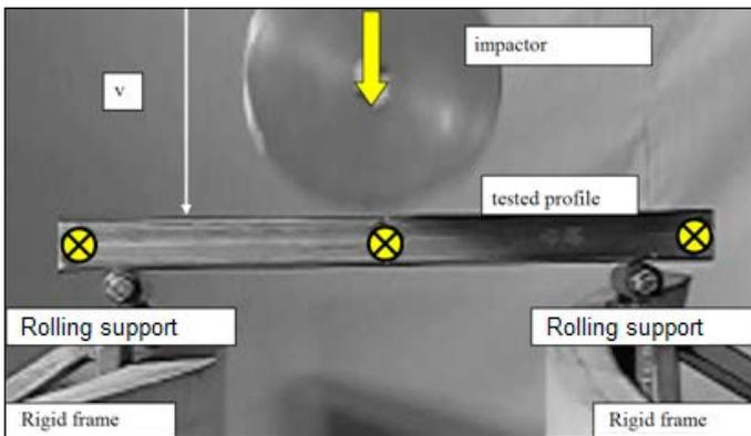
**FIGURE 4:** Drop test physical and virtual representation
