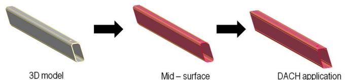
**FIGURE 6:** Pillar FEM model preparations
